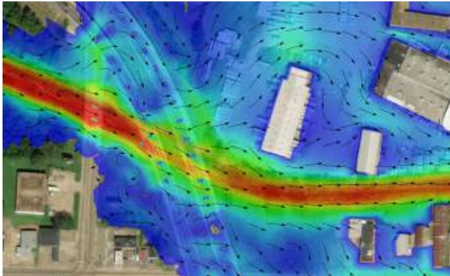
*Figure 730: Example of 2D Modeling<sup>6</sup>*
