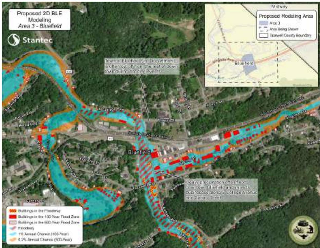
Figure 733: Bluefield Flooding Hotspots and Proposed Modeling Area
