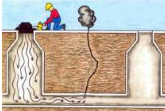
Figure 721: Smoke testing for I/5<sup>5</sup>
