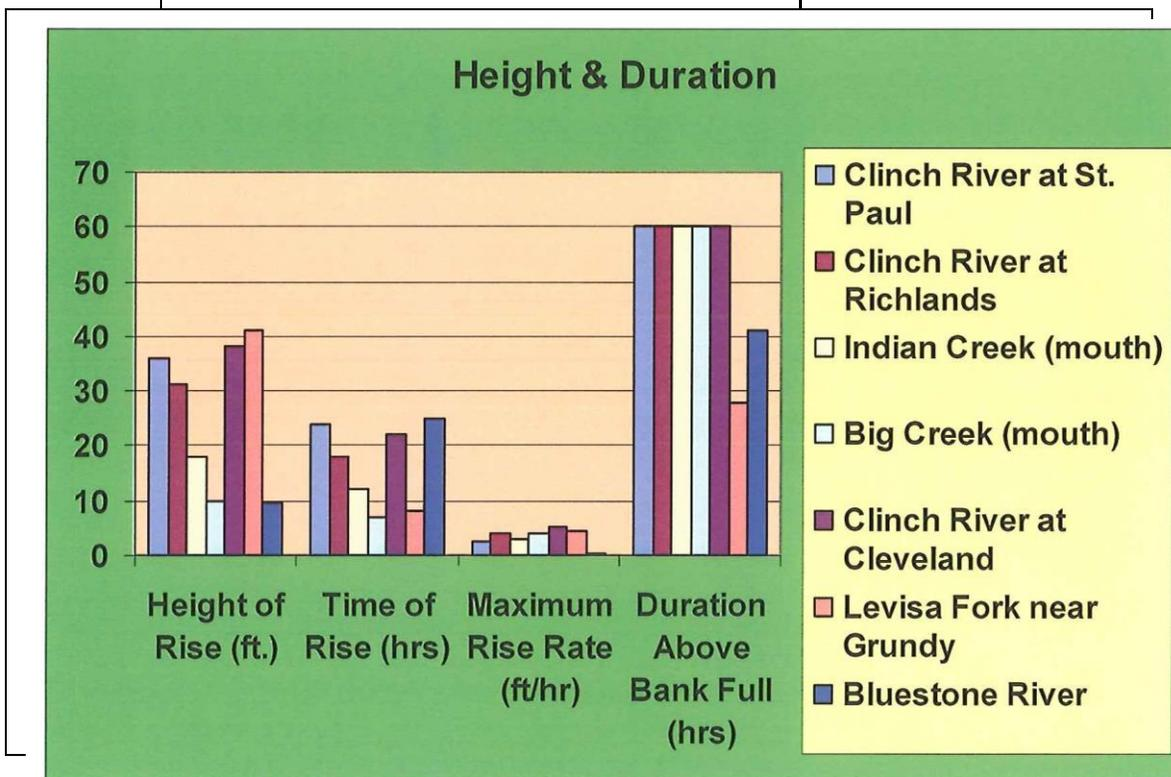
**Figure V-4 — River Basin Flood Heights and Duration**
