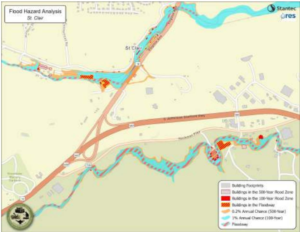
Figure 638: Flood Hazard Analysis – St. Clair Area
